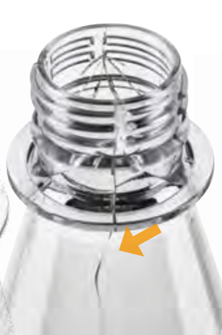
Cracks in the finish area
