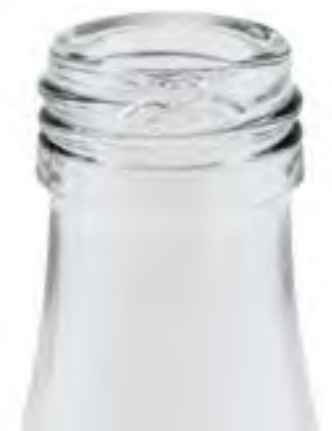
Damage in thread
