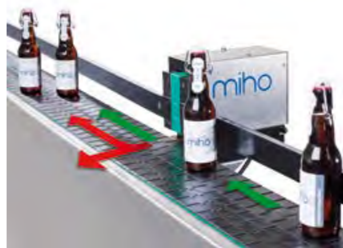
miho HSPM: multiple rejection (red arrows), depending on the type of bottle defect
