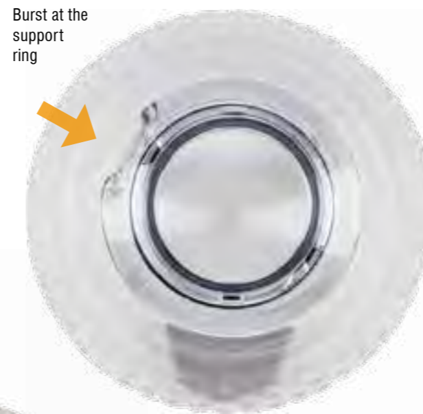
PET bottle: stress cracks, resulting in leakage
