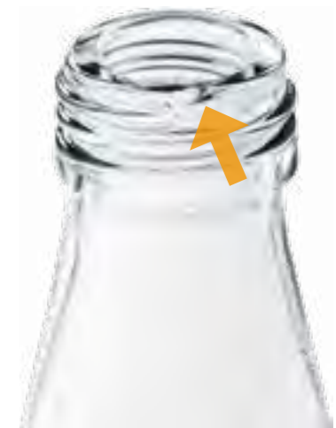
Glass: chip on the sealing surface
