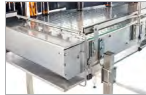
Reject table, with belt lubrication, height-adjustable foot receptacle and optional drip tray
