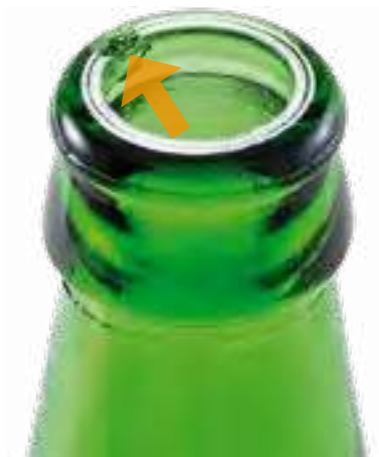
Glass: chip on the sealing surface
