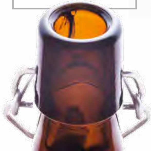
Swing top bottle with vertical split in the finish area
