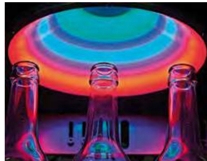
Sealing surface inspection with RGB lighting
