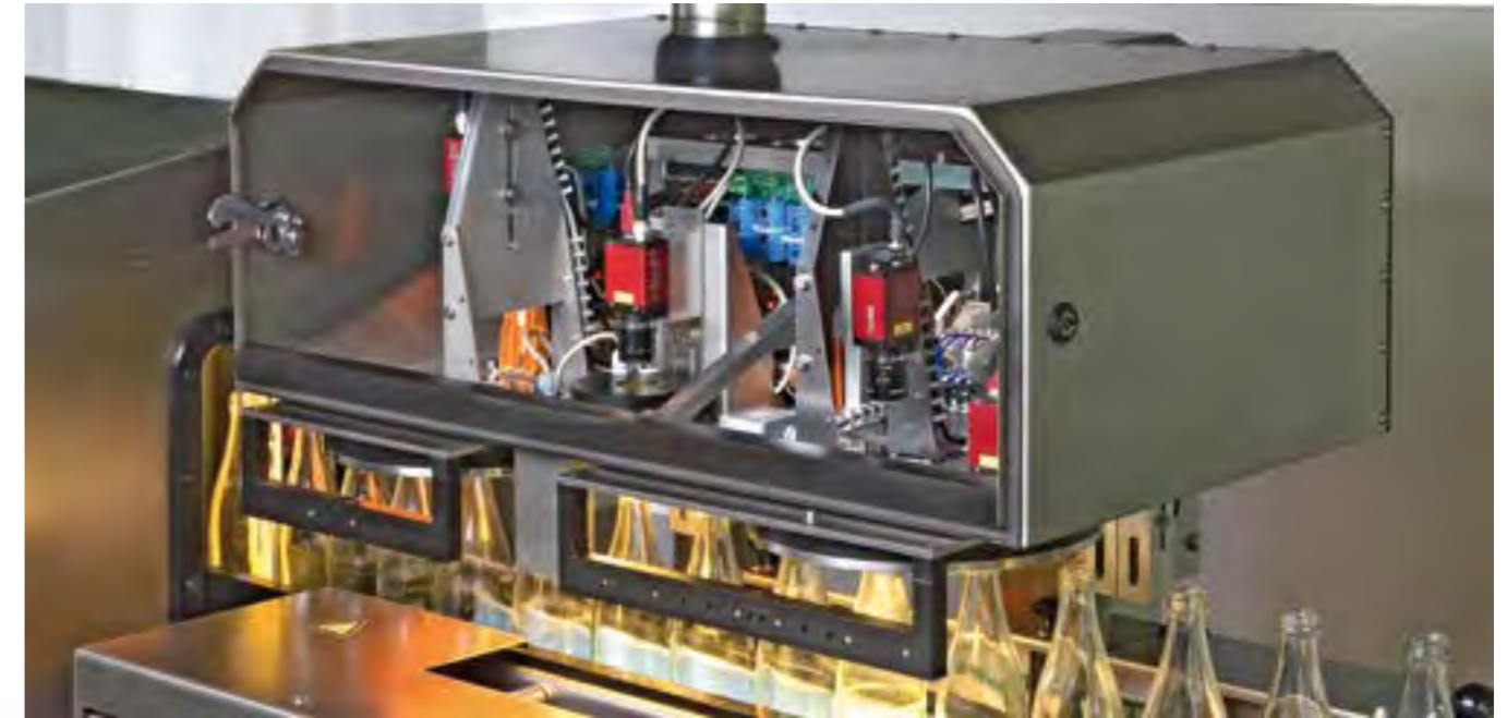
Inspection head of the basic machine, opened
