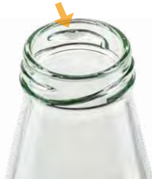
Twist-Off: Thread defect
