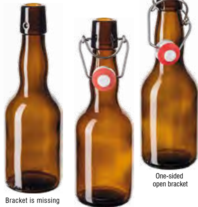
Bracket mounted the wrong way round
