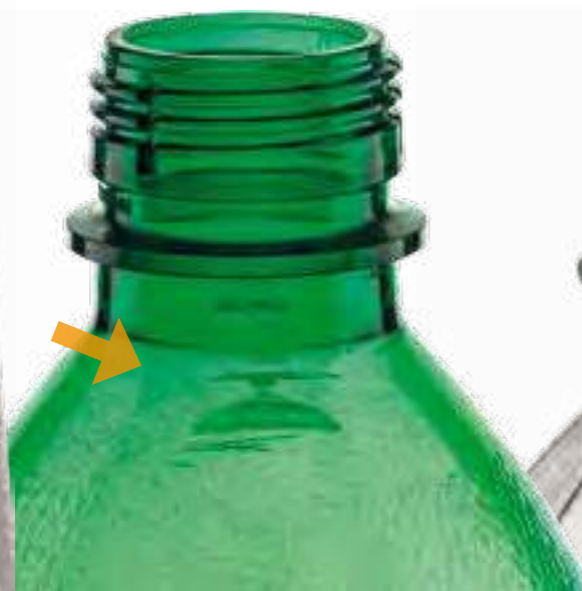
Abrasion through faulty neck ring guide
