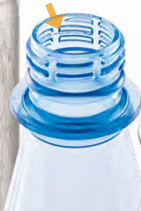
Damage in the threaded area
