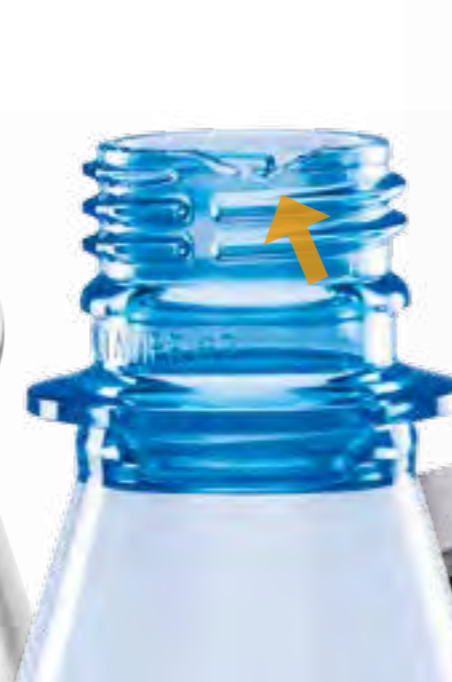
Burst at the sealing surface / thread
