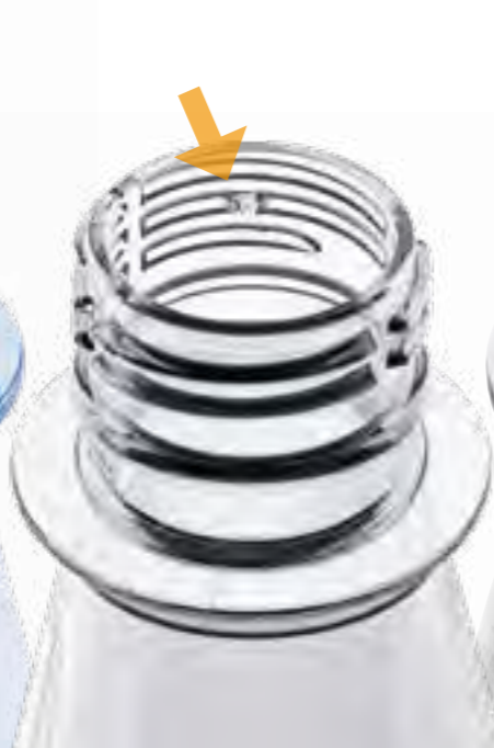
Damage to the thread
